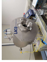
Figure 7: TVAC used for environmental testing
