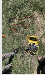
Soil Resistance Testing in North Field
